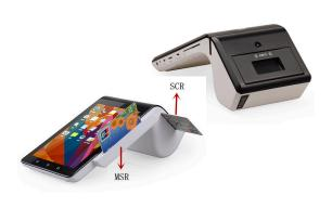
POS Station as Small Desktop Device Chip, Stripe and NFC Card Readers built-in Thermal Printer built-in (Receipts printed) Consumers pay using Cards or BIX Wallet Financial Transactions using Bank Accounts Limited Inventory / Sales Functions Administrative Functions using Web Portal
